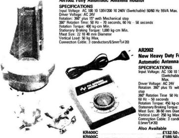
AR1002 Fully Automatic Antenna Rotator
